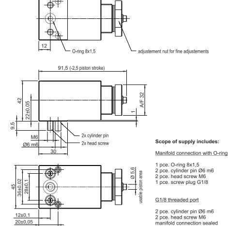
Pressure monitoring cylinder: Manifold connection with O-ring, bottom side G1/8 threaded port, back side O-ring 8x1,5 (spare part)
